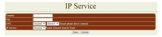
IP Server gives the user the ability to easily search for the name of the device other than searching for a long IP number. This flexibility allows the user to easily just remember the name of their device so they can access it with ease.
