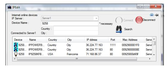
By setting the server address in IP server of advanced setup page, the user can easily search for his/her IP Power 9258-1U on internet just by searching for the name of the device. The **default IP address of IP server is 220.135.169.136.**
