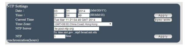
NTP synchronization : User can setup the time gap (  $1\sim300$  hours ) for 9258W2 to check the time with the NET server .
