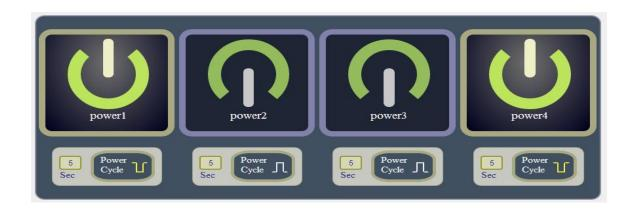
The following 3 pictures shows that after press the power cycle with 5 seconds setting , the outlet "Power1" will to turn off for 5 seconds and then turn ON . The power cycle action will execute after press the "Power Cycle" button .
