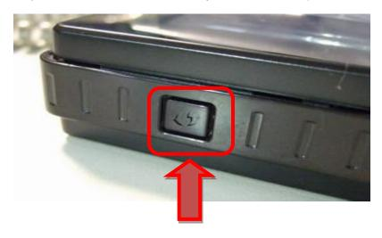
Step 3: Press One time ( short) the "Reset button" of 9258W2 and then there is one long beep which means the WPS function of 9258W2 enable.
