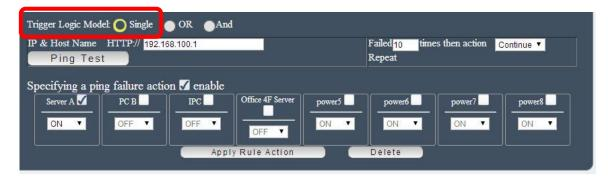
OR: 9258W2 will Ping 2 IP address. Either one IP fail times up to the setting times. Action (ON/OFF/RESET) will be activated.
