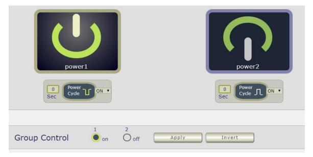
The following 3 pictures shows that after press the power cycle with 5 seconds setting , the outlet " Power1 " will turn off for 5 seconds , then turn ON later . The power cycle action will execute after press the " Power Cycle " button .
