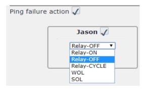
When the number of Ping Failures times have been reached. The device can be set to "ON, OFF, Reset-Cycle, WOL (Wake on Lan) & SOL (Shut On Lan) "function
