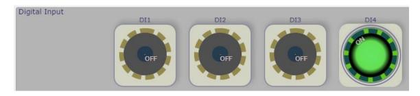
Note: We design the 4 standard DI for 9823 to use as all DRY contact or all Wet contact.
