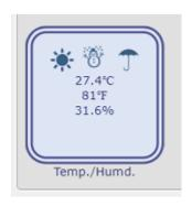
There is a Humidity & Temperature sensor on 9823GP-RL board shows the temperature value in Celsius (°C) and Fahrenheit (°F) and the Relative humidity (%)
