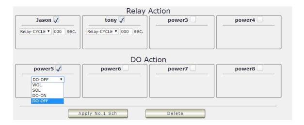
Once the scheduler has been Set Up , hit the "Apply No.X Sch" button and user will see user setting located on the bottom of the Action section .
