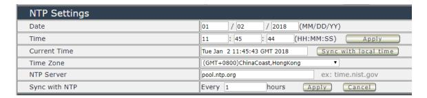
NTP synchronization: User can setup the time gap (  $1^{\sim}300$  hours ) for 9823 to check the time with the NET server.
