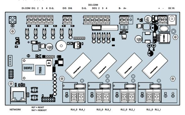
The system uses a plug-in screw terminal block for the interface between I/O modules and field devices. The following information must be considered when connecting electrical devices to I/O modules.
