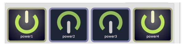
2 Power Cycle : Manually Control the relay delay some times to turn ON or OFF . The relay cycle time can be set from 1 to 9999 seconds
