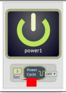
Original Outlet as "ON", select final status as "OFF "& fill 3 sec. After press "power cycle" button, the outlet will be ON for 3 seconds and then turn OFF.
