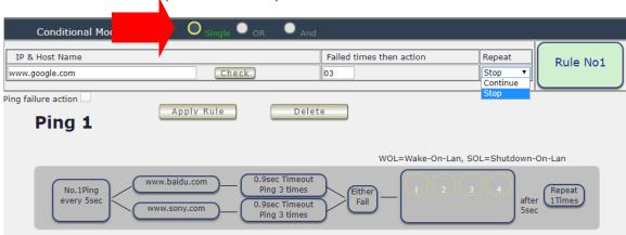
**OR**: 9820 MT will Ping 2 IP address. Either one IP fail times reach to the setting times. Action (ON/OFF/RESET) will be activated.
