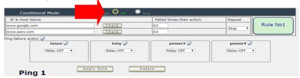
IP & Host Name: Input the IP Address (ex: 122.116.123.138) or Host - web address
