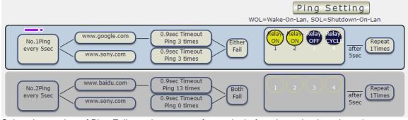
Select the number of Ping Failures that user prefer to do before the action is activated.
