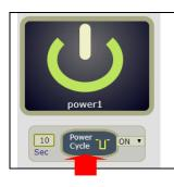
Original Outlet as "ON ", select final status as "ON " & fill 10sec. After press "power cycle" button, the outlet will turn OFF for 10 seconds and then turn ON.
