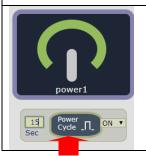
Original Outlet as "OFF", select final status as "ON "& fill 15sec. After press "power cycle" button, the outlet will turn OFF for 15 seconds and then turn ON.
