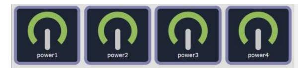
A-2 Power Cycle control: Manually Control the relay delay to turn ON / OFF. The relay cycle time can be set from 1 to 9999 seconds
