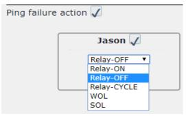
When the number of Ping Failures times have been reached. The device can be set to "ON, OFF, Reset-Cycle, WOL (Wake on Lan) & SOL (Shut On Lan) "function
